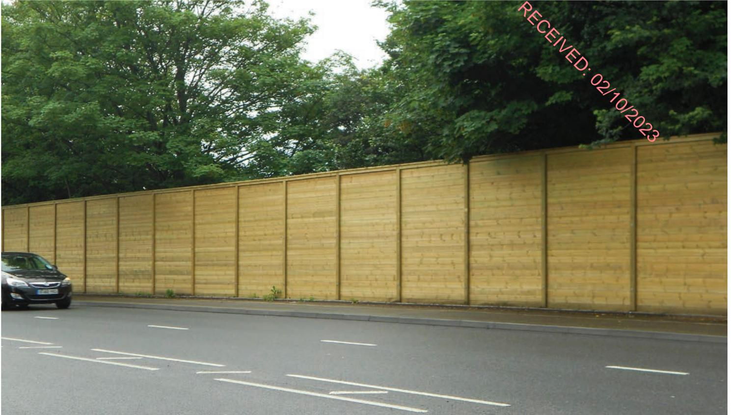
The Jakoustic® reflective barrier reflects the noise away using heavy section planed timber boards with a special profile that has been carefully developed. Boards are constructed in such a way that eliminates gaps that sound can easily travel through. Up to 28 dB\* in noise reduction.
